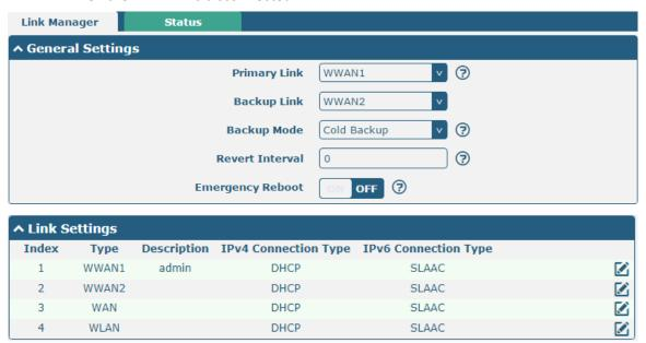
Click the button of WWAN1 to set its parameters according to the current ISP.
