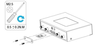
Insert or remove the SIM card as shown in the following steps.
