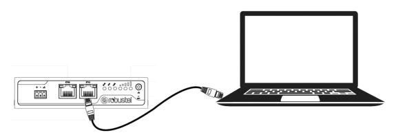
Connect an Ethernet cable to the port marked ETH0 or ETH1 at the bottom of the router, and connect the other end of the cable to your computer.
