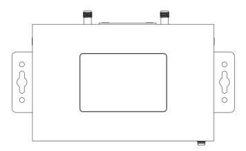
Use 4 pcs of M2.5\*4 flat head Phillips screws to fix the wall mounting kit to the router, and then use 2 pcs of M3 drywall screws to mount the router associated with the wall mounting kit on the wall.
