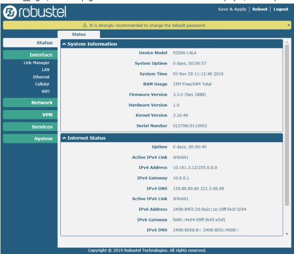
From the homepage, users can perform operations such as saving the configuration, restarting the router, and logging out.
