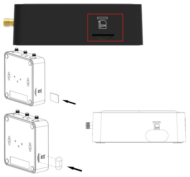
Insert or remove the SIM card as shown in the following steps.
